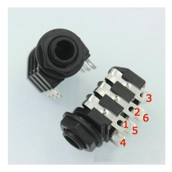
Pins 2-3 and 5-6 are joined so that it provides a mono signal to stereo headphones.
