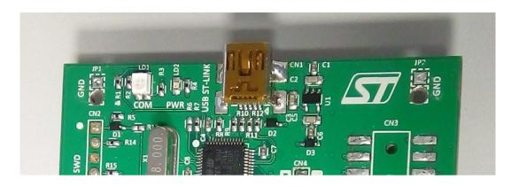
These holes should not cause the mounting screws to come into contact with any signals besides GND. To be extra safe, use M2 nylon screws.
